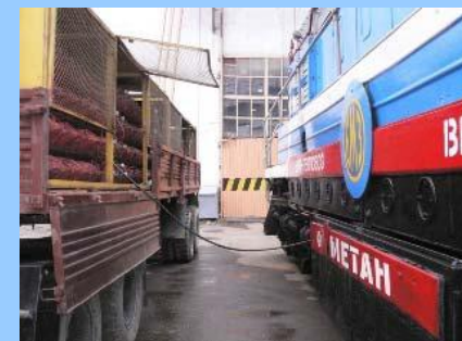
Natural Gas/Diesel Locomotive filled with LNG
