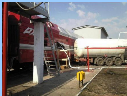
The GT-1 being filled with LNG
