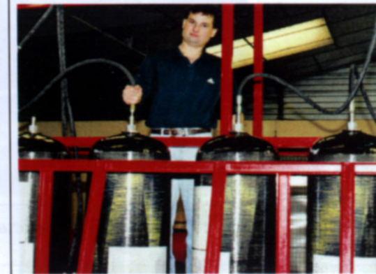
HYDRAULIC TEST PRESSURE 300 BAR
